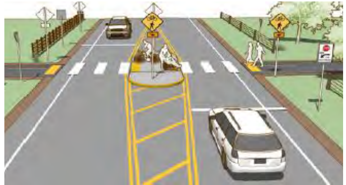
The proposed US 64B crosswalks at McClenahan St, Fayetteville St, Masonic St, and Small St all have space where median safety islands could be constructed, similar to the existing mid-block crossing along US 15/501 between Midway St and Launis St. See the Small Town and Rural Multimodal Network Design Guide pages 4-7 - 4-8 for further guidance ( ruraldesignguide.com ).
